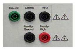
There are two monitor outputs on the Generator. These should be connected to the oscilloscope for monitoring the applied pulse. Connection to the oscilloscope should use a 100:1 probe with a minimum voltage rating of 1000 V. The monitor outputs are directly connected to the main outputs.
